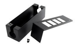
The FI Databox has a reversible lid, with a blanking plate on one end. The databox itself has a 25mm gland hole on one end and a 32mm gland hole on the other. Orient the lid to blank off one gland hole, leaving the required gland hole free.
